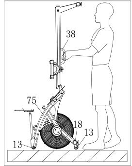
To move the machine, lift up the Rear supporter (46) until the transportation wheels on the Front stabilizer (18) touch the ground. With the wheels on the ground, you can transport the rower to the desired location with ease.
