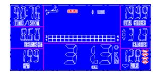
NOTE: When Rowing, the heart rate value depends on both of the sports loads and speeds. Heart rate controlling program is to keep the heart rate at the setting value. When the heart rate value measured during rowing is bigger than the set one, the loads resistance will decrease automatically, or the user slow down to lower the heart rate, whereas, the loads resistance will increase automatically or the user speed up to increase the heart rate.
